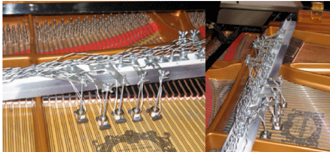
Figure 2. Electromagnets in a grand piano
